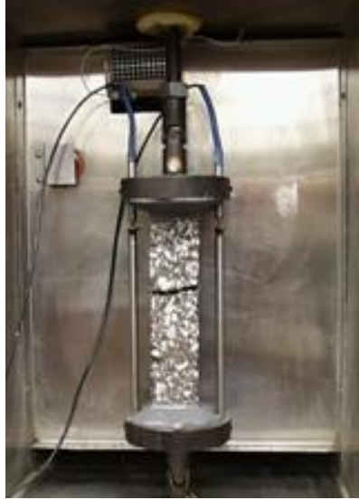
Figure 2-8. TSRST Test Configuration (Asphalt Research Consortium, 2007)
